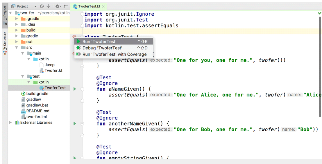
Figure A.5 Running the tests
