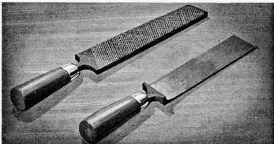
SCRAPER MADE FROM FILE
