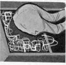
Wiggle the wires to see if solder has come loose.
