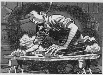
2. Sandpapering. The success or failure of a piece very often depends on the sanding. In order to work gradually up to the smoothest finish, start with grit size No. 1/0 and work up to grit size No. 2/0. Then go to next finer grit size No. 3/0 and thence to an even finer grit size of 4/0.
