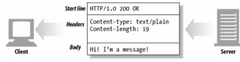
Figure 3-3. Three parts of an HTTP message
