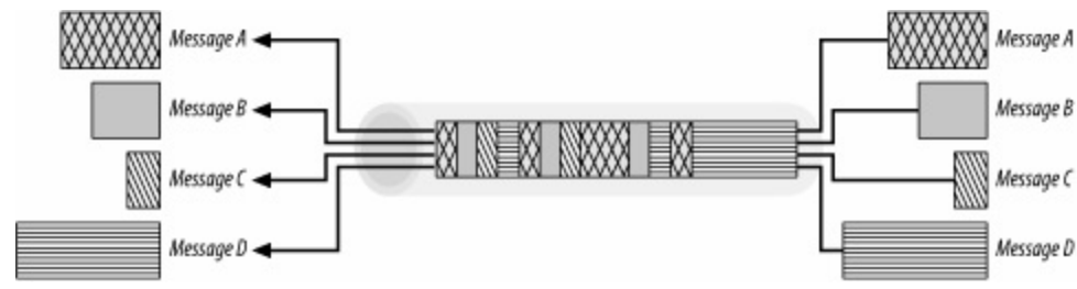
Figure 10-2. WebMUX can multiplex multiple messages over a single connection
