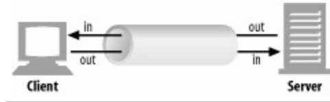
Figure 4-19. TCP connections are bidirectional
