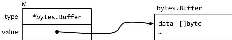
Figure 7.3. An interface value containing a *bytes.Buffer pointer.
