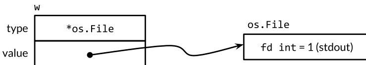
Figure 7.2. An interface value containing an *os.File pointer.
