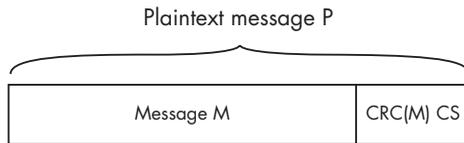
Now, the plaintext message needs to be encrypted. This is done using RC4, which is a stream cipher. This cipher, initialized with a seed value, can generate a keystream, which is just an arbitrarily long stream of pseudo-random bytes. WEP uses an initialization vector (IV) for the seed value. The IV consists of 24 bits generated for each packet. Some older WEP implementations simply use sequential values for the IV, while others use some form of pseudo-randomizer.
