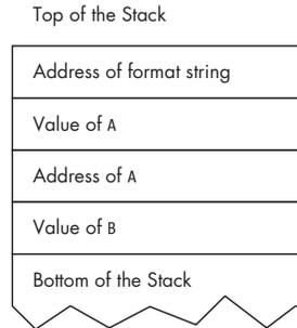
But what if only two arguments are pushed to the stack with a format string that uses three format parameters? Try removing the last argument from the `printf()` line for the stack example so it matches the line shown below.
