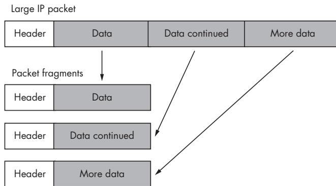
The packet is broken up into smaller packet fragments that can pass through the network link, IP headers are put on each fragment, and they’re sent off. Each fragment has a different fragment offset value, which is stored in the header. When the destination receives these fragments, the offset values are used to reassemble the original IP packet.
