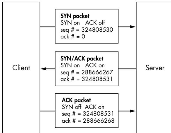
Sequence numbers allow TCP to put unordered packets back into order, to determine whether packets are missing, and to prevent mixing up packets from other connections.
