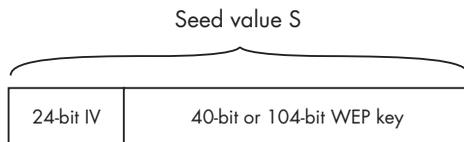
Then the seed value *S* is fed into RC4, which will generate a keystream. This keystream is XORed with the plaintext message *P* to produce the ciphertext *C*. The IV is prepended to the ciphertext, and the whole thing is encapsulated with yet another header and sent out over the radio link.
