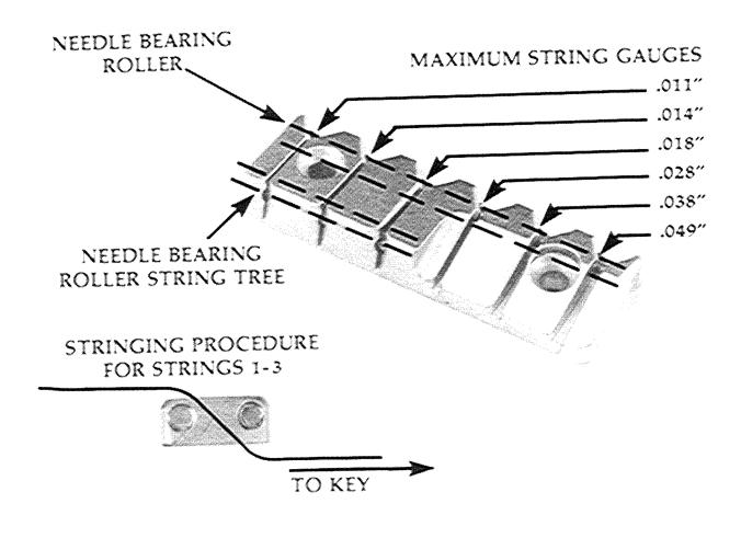
and locking keys. However, since the optimum height adjustment varies from player to player due to differences in technique, playing styles, string gauges, etc., additional precision-rolled, stainless steel shims are available (.010", .005", .002") to adjust the roller nut height for your playing preference.
