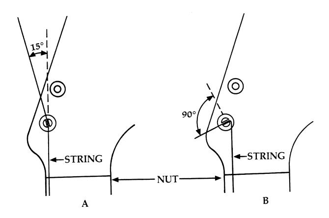
Be sure the string hole in the string post is at approximately 15° (A) to the left of a line perpendicular to the nut. Draw the string through the hole, tautly, and lock in place by turning the String Locking Button clockwise. Then turn the key until the string hole rotates counterclockwise approximately 90° (B). Tune to pitch.
